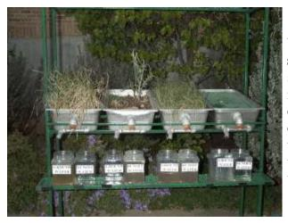
What is a Rainfall Simulator? A **rainfall simulator** simulates a rainfall event on a small specific area and allows water to either soak into the ground, through a porous soil layer and drain out the lower holes and into the container called :ground water"; or it runs off the top of the soil surface or impervious layer and out the top hole spilling into the container called "runoff water".
